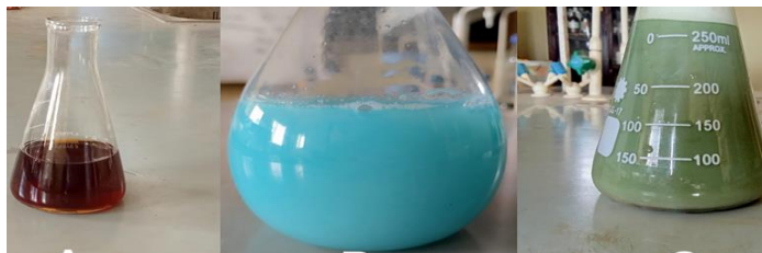
Plate 1: (a) Hierochloe odorata aqueous leaves extract (b) AgNO 3 & CuCl 2 salt solution (c) solution of Ag-Cu nanoparticle
