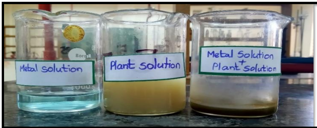
Figure 3: Beakers containing copper sulphate solution, orange seed extract and synthesized copper nanoparticles
