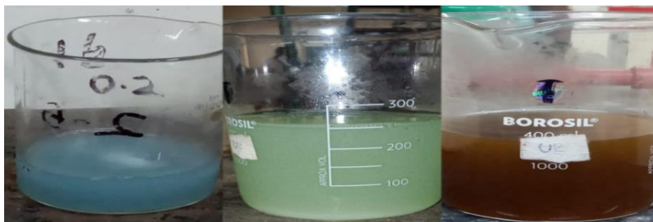
Figure 6: Colour changes from blue to dark brown after adding citrus sinensis extract
