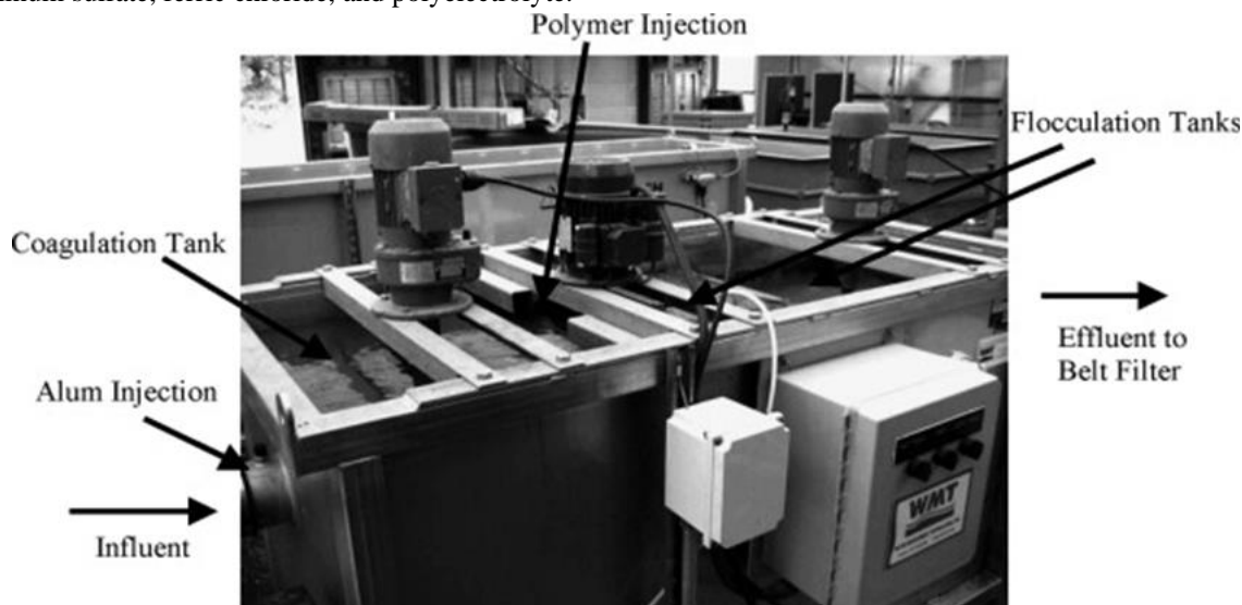
Figure 3: The coagulation/flocculation tank with two variable speed mixers
