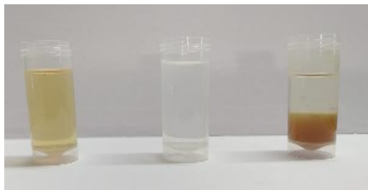
Figure 3: Test tubes from left: Aqueous PG Stem extract, Zinc Acetate solution and Synthesized ZnNPs
