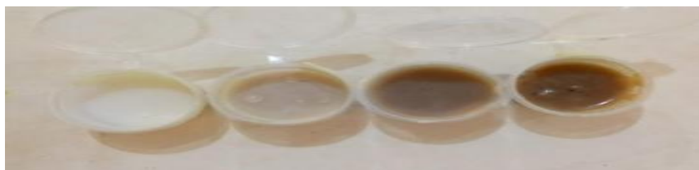
Figure 2: Four soaps prepared (i.e. in the ratio CNO:MKO); 100:0, 80: 20, 50:50, and 0:100, respectively from left to right
