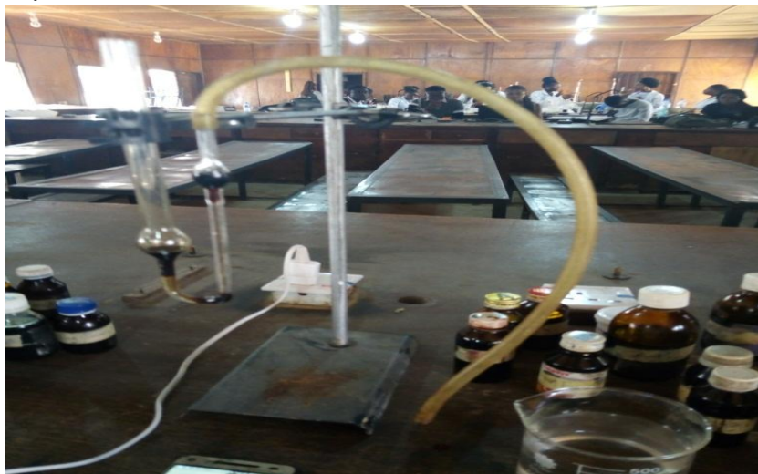
Plate 4: Using the U tube Viscometer to Measure Viscosity of the Lube Oil
