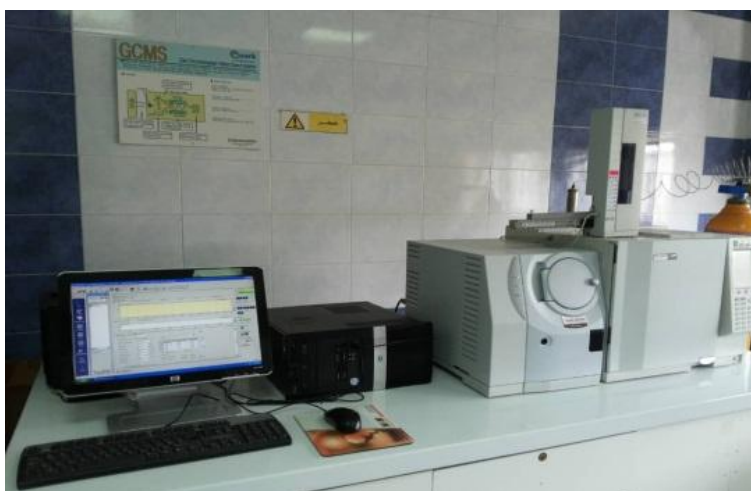
Figure 1: Gas Chromatography system equipped with Mass Spectrometry detect
