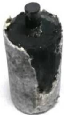
Figure 2: The internal content of the spent (Zn-C) battery
