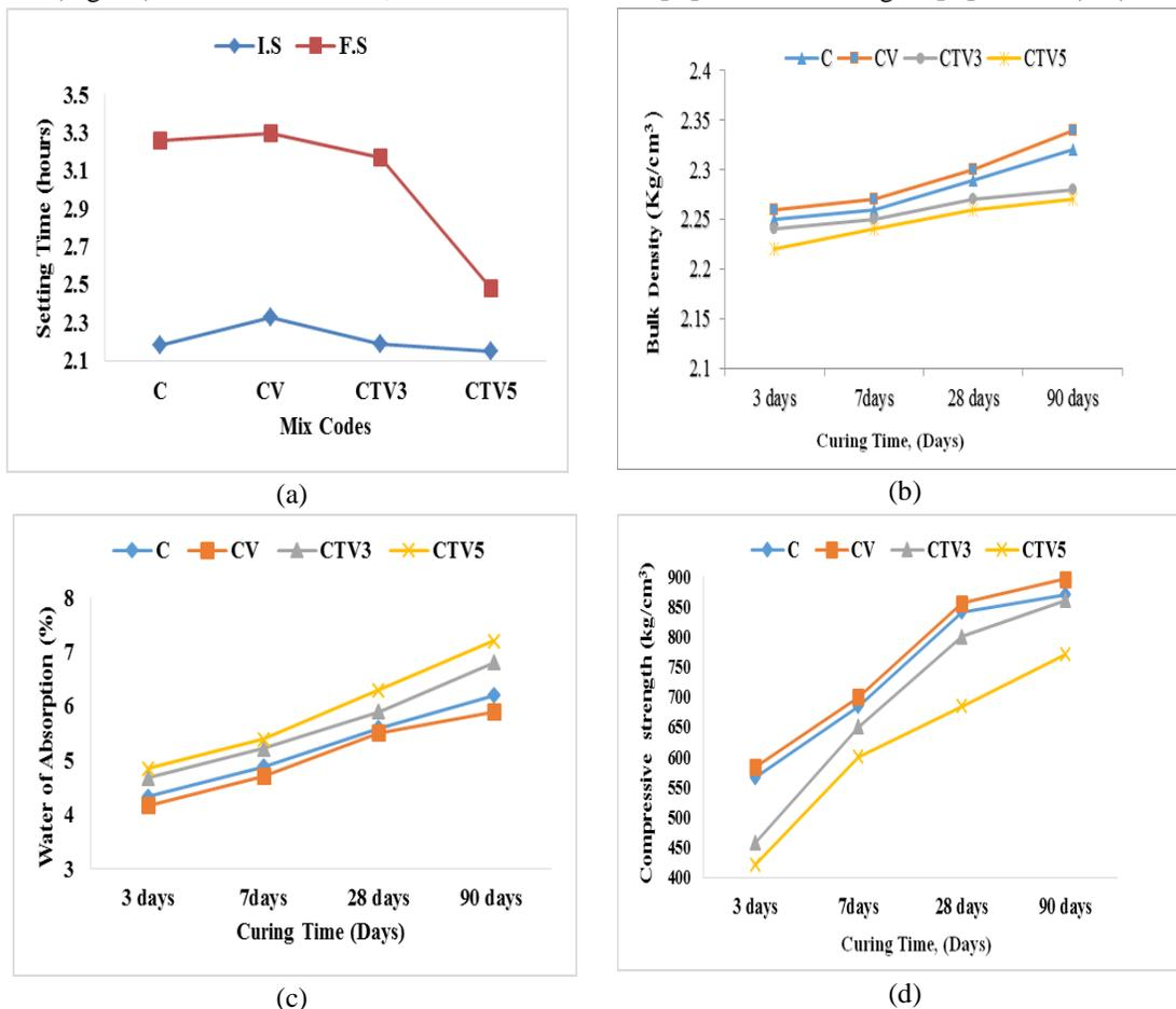
Figure 5: a) Initial and final setting times; b) Bulk density; c) Water absorption; d) Compressive strength of different mixes
