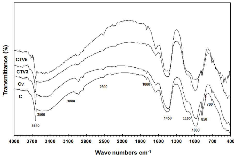
Figure 4: FTIR spectra of the studied mixes cured for 3 months
