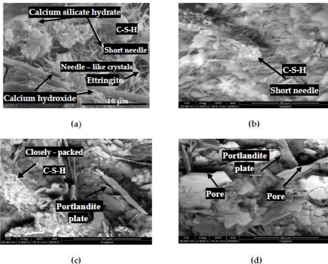
Figure 3: SEM images of hardened cubes of the studied mixes cured for 3 months a) C mix; (b) CV mix; (c) CVT3; (d) CVT5 mix.
