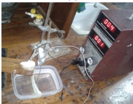
Figure 9: Set up used to test the permeability of chitosan film for Cd(II) under an external power supply
