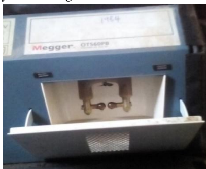
Figure 1: Megger transformer oil tester, showing the electrodes
