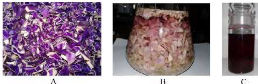
Figure 3: The major steps of the process of extraction of red cabbage, A: red cabbage pieces, B: extraction with ethanol, C: final anthocyanin extract.
