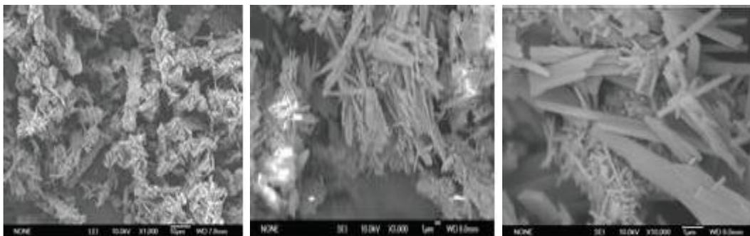
Figure 15: FE-SEM micrograph of zinc oxide synthesized in different magnification
