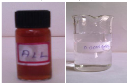
Figure 2: (a) 0.001 N Silver nitrate solution, (b) silver nanoparticles after addition of extract
